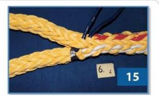
J. The splice is now finished. Tape the two most close laying ends together (if the procedure has been followed correctly then such a pair will consists out of a left and right hand laid strand) and cut off the over length
