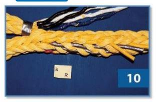
G. The fourth pair (4L, left, black), go under resp. the 1st and 2nd strands of the body (calculated from the tucks made at F) Then follow same procedure  $\frac{11+12}{1}$ .
