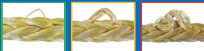
Pulled yarns protruding from rope surface: single yarn (left), partial strand (middle), strand (right)
