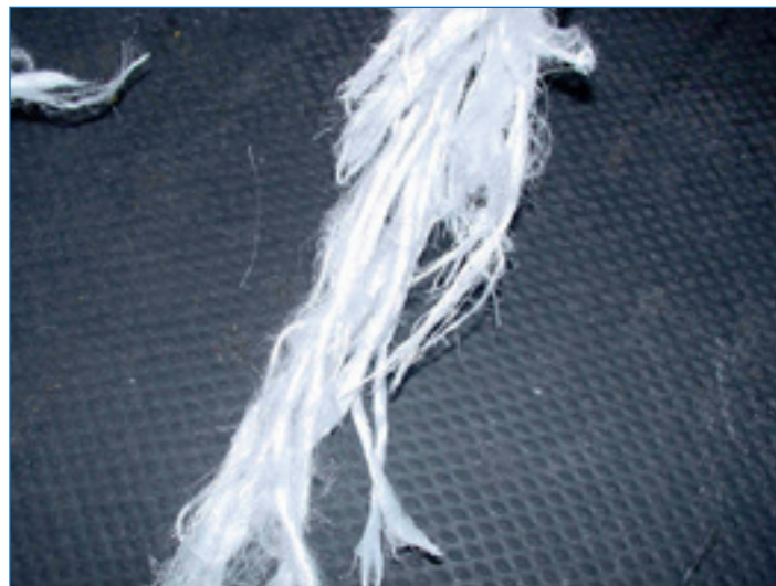
Broken due to overload (rope must be rejected)
