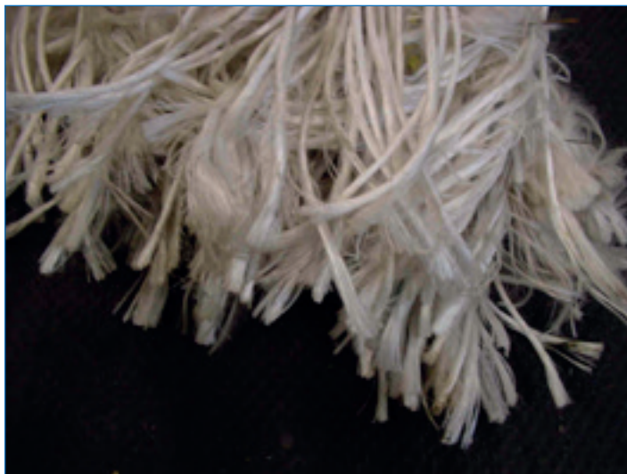
Broken on sharp edge (this rope can be re-spliced)
