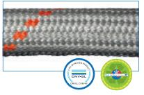
STRONGLINE™ has a rope construction comprising a parallel core with a braided protective cover. The parallel core produces a far higher strength rope than might be expected for a rope of this diameter and material. The protective cover ensures a long service life due to its excellent resistance against abrasion. Regular maintenance can significantly lengthen the rope service life. The main applications of STRONGLINE $^{\text{TM}}$  are towing and mooring.
