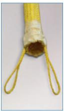
A high performance protection sleeve for permanent fixing on a hawser, towing line or pennant. The braided strands offer high abrasion resistance. The sleeve is made in a hollow braid, and can be easily be adjusted to the circumferential size of the rope being protected. The DEFENDER® can be made from different types of yarns, offering extra strength, floatability and other characteristics. Please consult our sales staff for the optimal product in your application.
