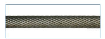
Multi strand, non-rotating, hoisting wire rope. During the LANKO®LIFT COMPACTED production process, the core is covered by an especially designed HDPE extruded cover. This special feature gives the wire rope stability, and avoids pointto-point contact between wires of the outer and inner strands, as well as preventing corrosion and wear of the core. When the high breaking strength is taken into account, this hoisting wire rope offers exceptional quality.
