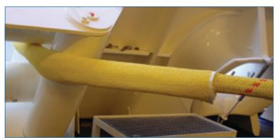
If the rope is affected by rough surfaces or sharp edges, it can be easily damaged. Also in case of high abrasion resistance, high cut-resistance and high chemical resistance protection of the rope is needed. Lankhorst Ropes provide innovative high performance protection solutions to prevent loss of strength and maximize the life of the fi bre rope. Please consult our sales departments for the optimal sleeve to use in your application.
