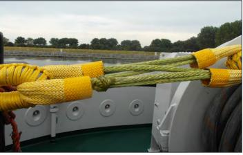
direct connections between polyester/HMPE lines where the ropes will cut through.
