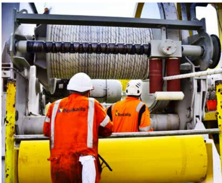
A Lankoforce with Dyneema jacket onboard a vessel
