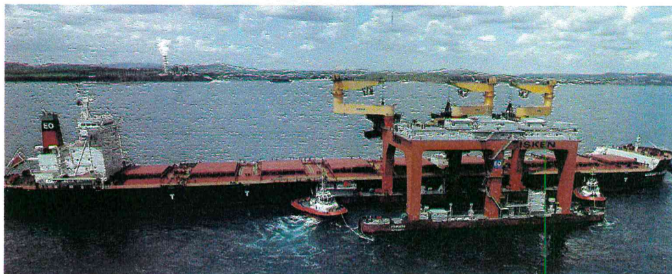
◀ Tugs bring the Transshipper Isken alongside a coal carrier in the Bay of Iskenderun in southern Turkey
