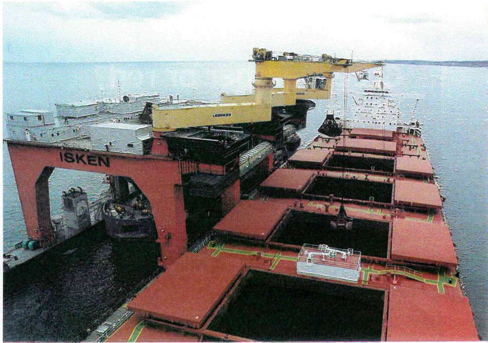
▲ Transshipper Isken unloads coal from a carrier on to a self-unloading barge
