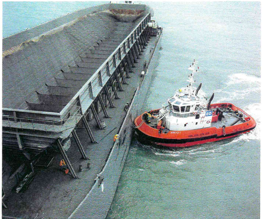
▲ A self-unloading barge is assisted into place during the coal transfer operation
