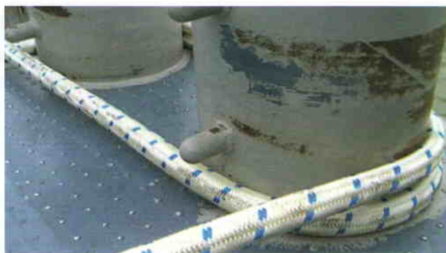
New synthetic rope specifically for connecting container barges for inland duties.
